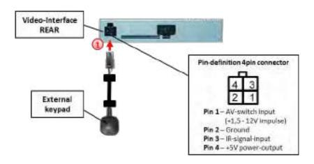
Connect 4pin female Microfit connector of external keypad to male 4pin Microfit connector of video interface
