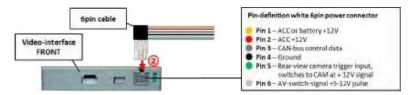
Connect white female 6pin Molex connector of the 6pin to 8pin cable to the male 6pin Molex connector of the video-interface.
