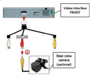
1 Connect the video-RCA of the after-market rear-view camera to the female RCA port of the video-interface which is labeled as CAM.
