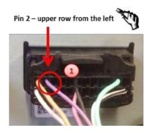
① Cut the cable at pin 2 of the upper row from the left side and isolate both ends.
