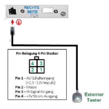
Onnect the keypad's female 4pin connector to the video-interface's male 4pin connector.
